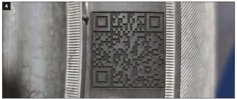
Figure 4: The QR code (mirrored) engraving on the sidewall of the Barez tire using a fiber laser
